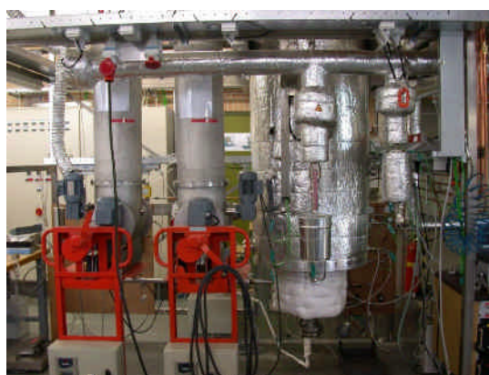
Figure 3. Lab-scale 5 kg/h Milena indirect gasification reactor at ECN
